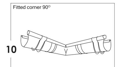
A correctly placed corner does not need to be supported by a hanger
